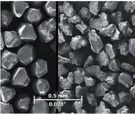
**Figure 3.** Blocky (left) vs. angular-shaped grains.
