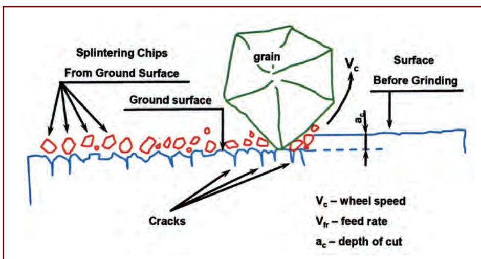
**Figure 1.** Material removal mechanism.
