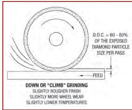
**Figure 4.** Schematic of the depth of cut.
